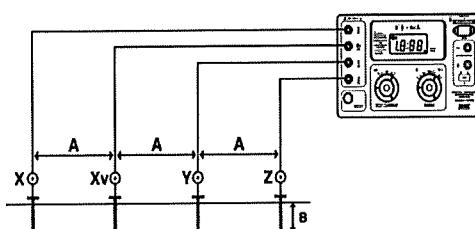
Electrode Spacing (A) [ ] cm      Electrode depth (B) [ ] 15 cm      B = A/20
