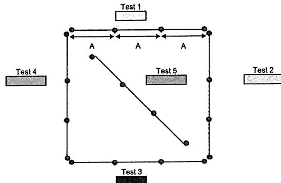
$$\rho \text{ calculation} \quad \rho = 6.283AR \quad \Omega \cdot \text{cm}$$
